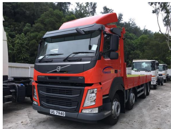
3 units of 4 axles 24 ton truck with lower platform
